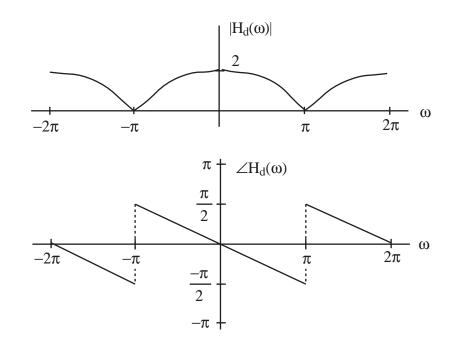
Here we do have jumps of  $\pi$  at  $\omega$  = odd multiples of  $\pi$ , but we will still call this linear phase.
