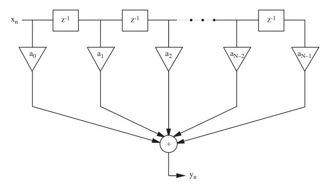
Due to the arrangement of the delays, this is also called a transversal filter or tapped delay-line filter.
