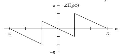
Summary: In this example,  $\angle H_d(\omega)$  is generalized linear phase but it is not linear phase.
