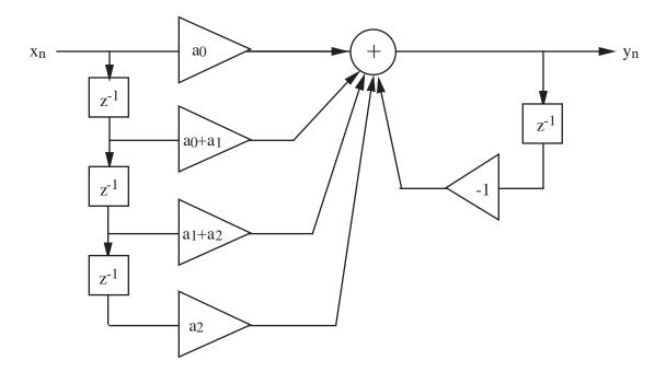
This is a recursive structure ( $y_n$  depends directly on  $y_{n-1}$ ) that realizes the transfer function H(z).
