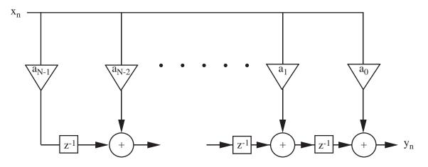
This structure has the same transfer function as the Direct Form structure and is very commonly used.
