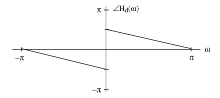
Since  $R(\omega)$  will be odd for any antisymmetric filter, we conclude that <u>filters with antisymmetric</u> <u>coefficients cannot have linear phase</u>.
