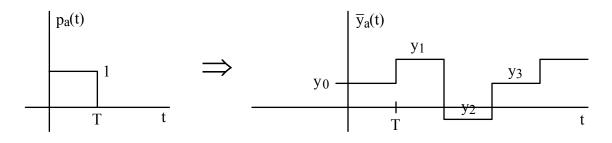
Thus, the ZOH output is a staircase approximation to the desired  $y_a(t)$ . This staircase must be smoothed by  $F_a(\Omega)$  to produce the proper  $y_a(t)$ .
