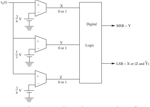
Here,  $0 \le x_s(t) < \frac{1}{4}$  is mapped to (0, 0),  $\frac{1}{4} \le x_s(t) < \frac{1}{2}$  is mapped to (0, 1),  $\frac{1}{2} \le x_s(t) < \frac{3}{4}$  is mapped to (1, 0), and  $x_s(t) \ge \frac{3}{4}$  is mapped to (1, 1).
