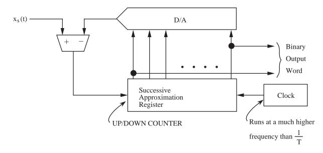
Here,  $x_s(t)$  is the input from the sample and hold. The above system quantizes  $x_s(t)$  to fit into a computer register. The comparator output signal causes the up-down counter to either increment or decrement, at a high rate, until it contains a binary approximation of  $x_s(t)$ . When the counter has settled around the correct digital representation of  $x_s(t)$ , it simply toggles back and forth in its least significant bit until the value of  $x_s(t)$  changes.
