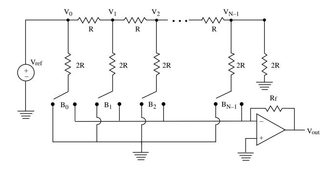
The switches are transistors, where the  $B_i$  control whether the transistors conduct to ground (left position,  $B_i = 0$ ) or to the op amp (right position,  $B_i = 1$ ). The op amp then adds all signals input to its minus terminal, with a weighting determined by the resistor values. To find the exact relationship between  $V_{out}$  and the  $B_i$ , first apply KCL at Node N–1 at the upper right, to give:
